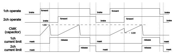
Figure 37. Current limit mask function timing chart
