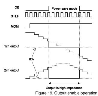
When the OE pin is set High, the output is forced OFF and goes to high impedance.
