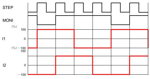
Figure 22. Current waveform of Full step in CLK-IN
