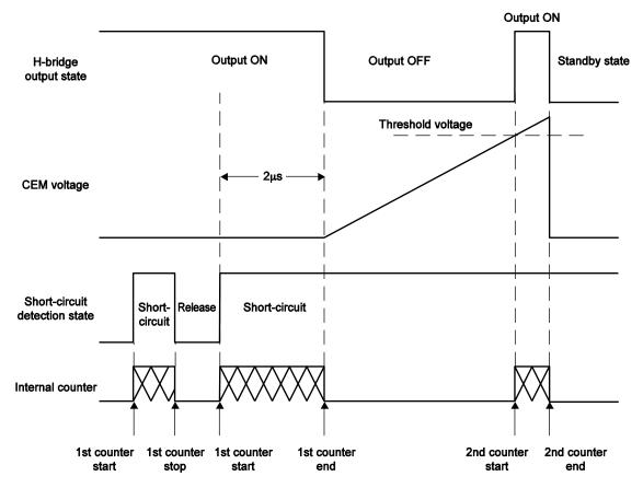
Figure 44. CEM operation timing chart in latch type
