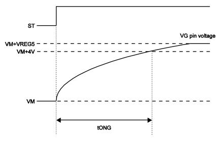
Figure 46. VG pin voltage schematic view
