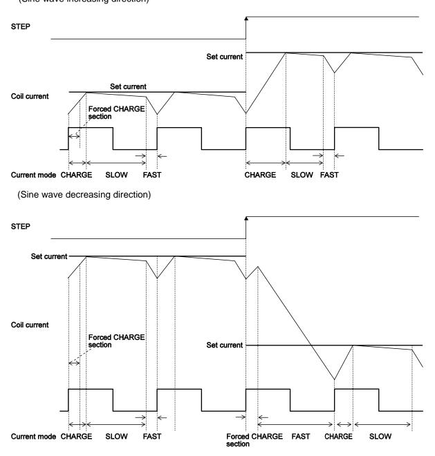
Figure 27. Current control operation
