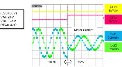
Figure 17. Attenuation operation
