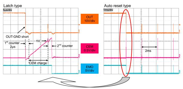
Figure 45. CEM operation waveform
