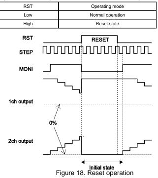
When the RST pin is set to High, the excitation position of the output is forcibly set to the initial state, and the MONI output is placed in the ON state. When RST is then set to Low, the excitation position is advanced by the next STEP input.
