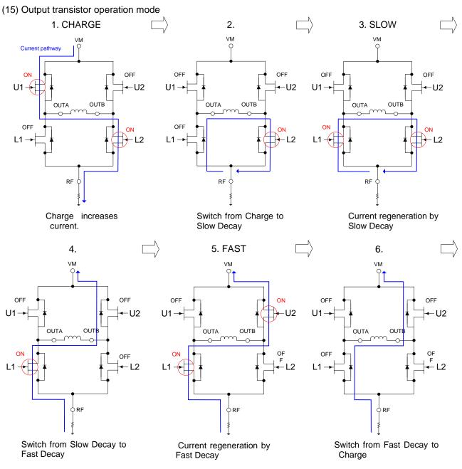
Figure 28. Switching operation
