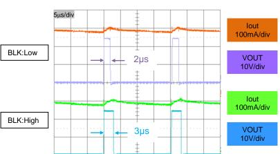
Figure 39. Blanking time waveform
