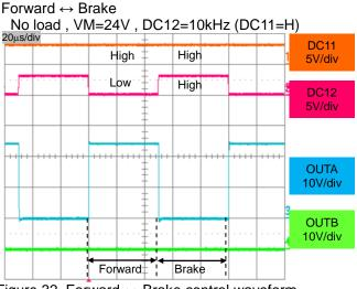
Figure 32. Forward ↔ Brake control waveform
