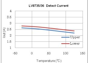
Figure 43. Detect current vs temperature
