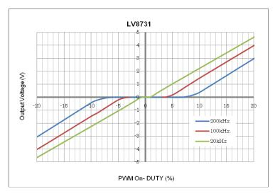
Figure 31. PWM control characteristic
