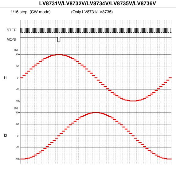
Figure 26. Current waveform of 1/16 step in CLK-IN
