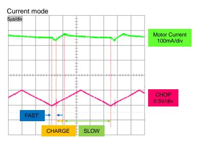
Figure 30. Chopping waveform
