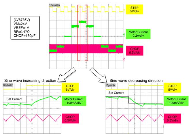
Figure 29. Current control operation waveform
