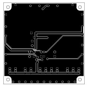
L2 : Copper wiring pattern diagram
